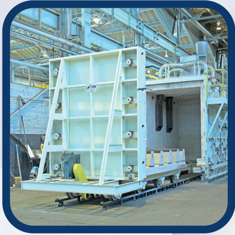
Car Bottom Furnace
