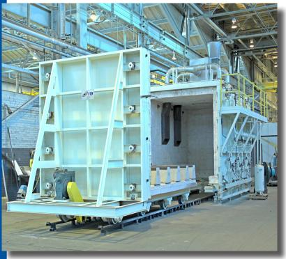
ITS Standard TruTemp<sup>™</sup> Car Bottom Furnaces are an excellent solution to process your large and heavy materials, from welded fabrications and forgings to spun products and plates.
