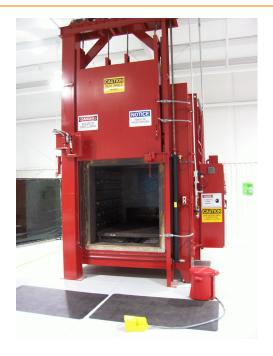
The TruTemp™ Box Furnaces are an excellent solution to heat treat a wide variety of materials, from welded fabrications and forgings, to spun products and plates. Processes include tempering, hardening, normalizing, annealing, preheating and stress relieving to name a few. Industries served are aerospace, oil drilling, steel mills, automotive, military and many more. Materials processed include aluminum, steel, cast iron, high nickel alloys, titanium and others.
