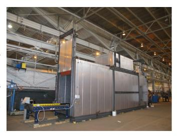
By comparison, a batch oven only allows for product to be placed in a static position for thermal processing. Depending on how the oven is used, product may be positioned consistently and uniformly inside of the chamber, or more often fairly randomly. While a batch oven can be more of a "one-size-fits-all" solution, it can produce varied results (within and between batches). Depending on the customer process, this may be perfectly acceptable.
