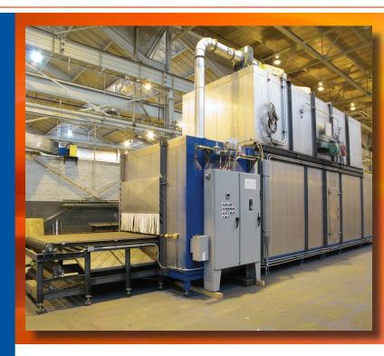
Core Wash Drying Ovens work with minimum heat absorption. The purpose of the Core Wash Drying Oven is to dry core wash coating applied to sand cores. The process will eliminate the space and time required for the ambient air drying of sand cores. Proper air circulation and exhaust sizing accelerates drying time and allows the cores to dry with minimum absorption of heat into the sand core.
