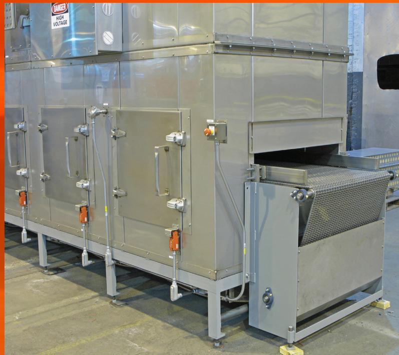
**Conveyor Oven handle high production rates. Loading product(s) into the oven can be manual or automated.**
