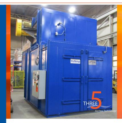
ITS offers out of autoclave composite curing ovens that provide the most economical, reliable solutions to meet your composite processing requirements.
