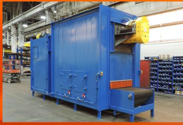
Conveyor ovens can be zoned based on a required temperature profile -- up to a zone for every profile segment. Further, a customer process may often dictate that their product must be cooled.
