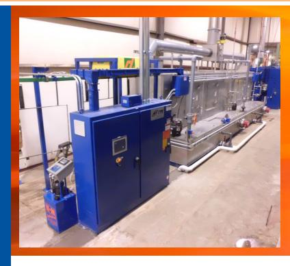
The Monorail Washer is a universal system serving a wide variety of OEM manufacturing applications. It is designed for mass production utilizing an overhead trolley monorail or powered conveyor.
