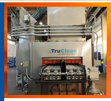
We offer single to multi-stage configurations, and can manufacture belt widths to exacting customer specifications with flat wire, balanced weave, mesh or various non-metallic materials handling designs and options for heat mediums include electric, gas, LPG or hot water and steam.
