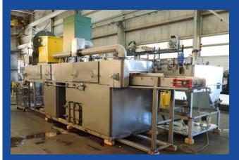
The washer features a conveyor that is 55" high vs. the standard 39".
