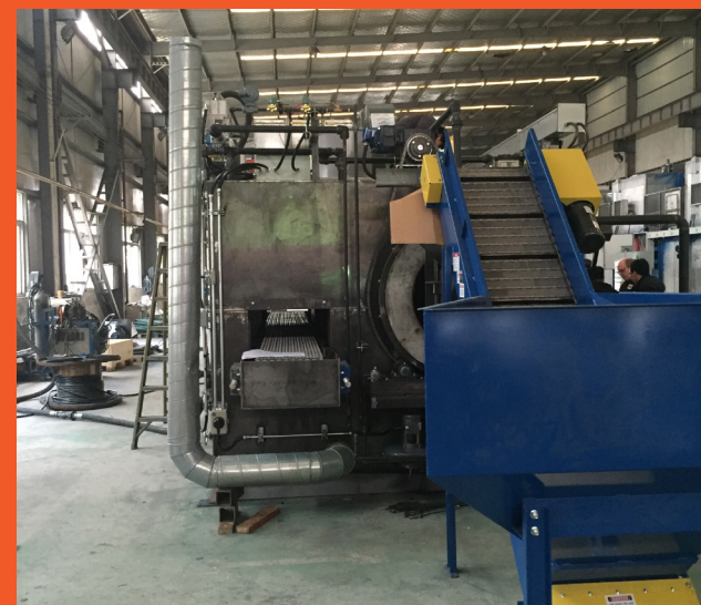
The washer features both a conveyor and a rotary drum.
