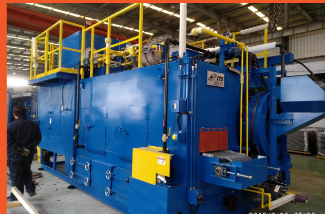
The washer features both a conveyor and a rotary drum.
